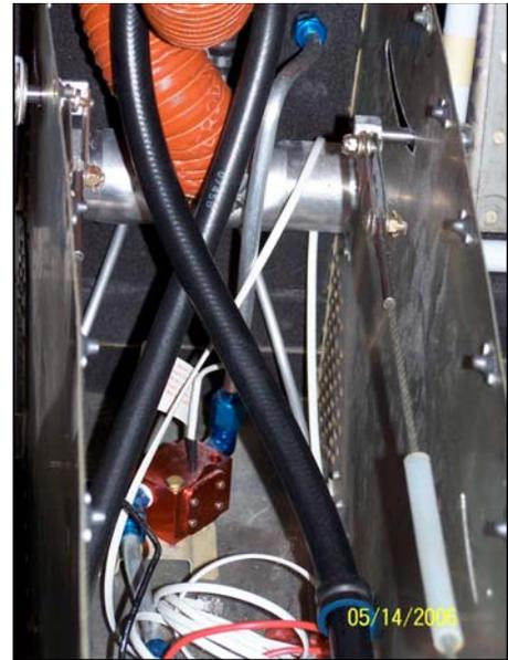
MS21919DG-xx clamps were used on the hose routing forward of the aft spar. I used MS21919DG13 clamps on the H-03 hose and MS21919DG-11 clamps on the H-04 hose. The hoses were routed along the bottom of the tunnel then angled up aft of the control tube and over the forward spar.
