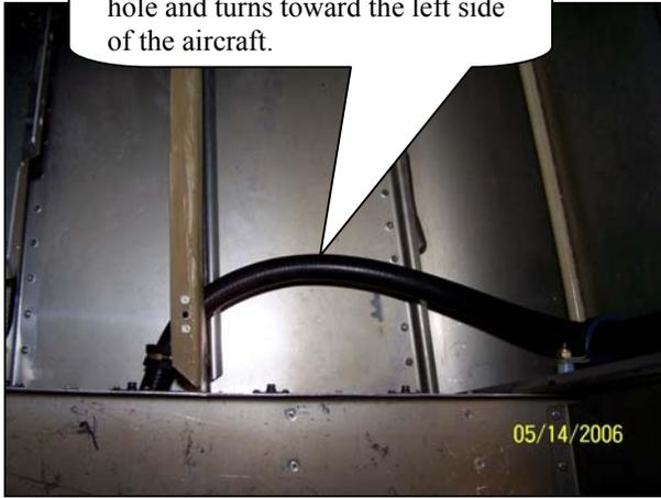
The H-03 hose goes up to the evaporator's top fitting. The hose is clamped to the F-1006 bulkhead assembly with MS21919DG-13 clamps.
