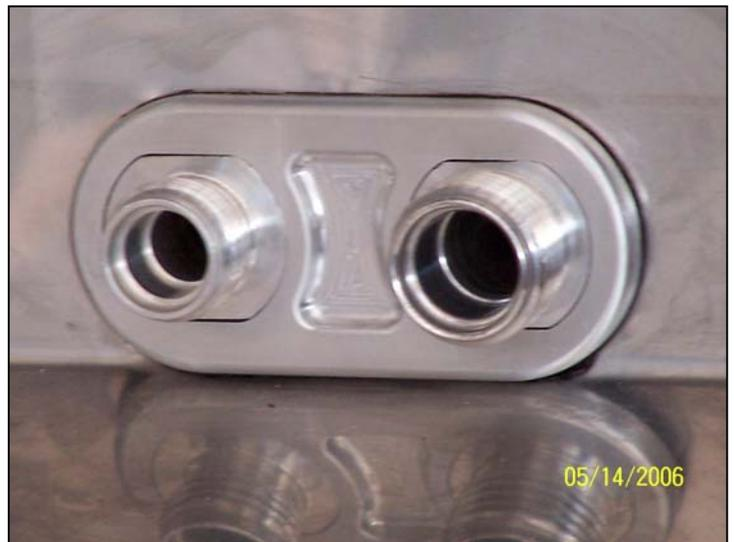
The 90-degree fittings attach to the back of the bulkhead fitting. The H-03 and H-04 hoses clear the forward cabin heater hose for and support and hold the aft cabin heat hose in the center of the tunnel. You may notice that the picture on the right shows the rudder cables running on the inside of the tunnel. This is a modification I made to my aircraft shown on this web site. The hose routing will clear the standard rudder cable routing also.
